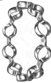
Fig. 52. Pressed-steel welded cage.
