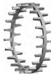
Fig. 44. One-piece, machined-brass, roller-riding, finger-type cage.
