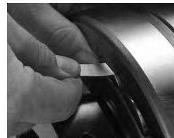
Fig. 95. Measure of RIC before installation.
