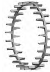
Fig. 45. One-piece, machined-brass, land-riding, finger-type cage.
