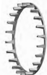
Fig. 46. Split, machined-brass, land-riding, finger-type cage.
