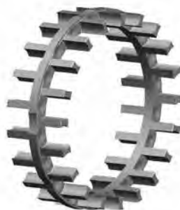
Fig. 49. One-piece finger-type cage.
