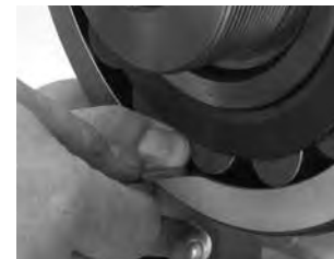
Fig. 92. During mounting, the RIC should be checked at the unloaded roller.
