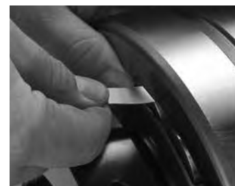
Fig. 95. Measure of RIC before installation.
