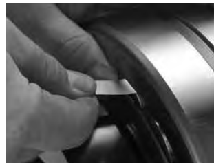
Fig. 91. Measure RIC before installation.
