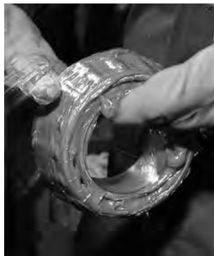
Fig. 147. Grease can easily be packed by hand.
